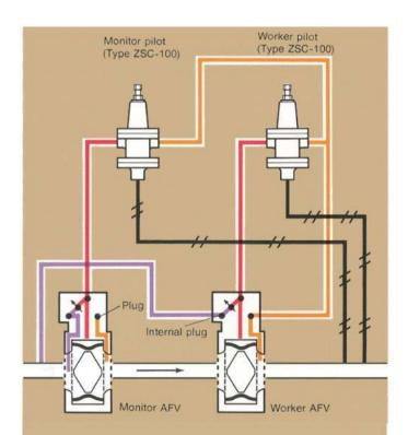
Pressure reduction with monitor. During normal operation, a single AVF, the worker, performs the pressure cut. The monitoring pilot is set at an output pressure slightly higher than the working pilot. Since the monitoring pilot is always open, the monitor AFV is held in the full open position. If a malfunction occurs on the worker side, the output pressure rises to the monitor setpoint and it assumes control. The roles of worker and monitor can be reversed by simply resetting the pilots.
