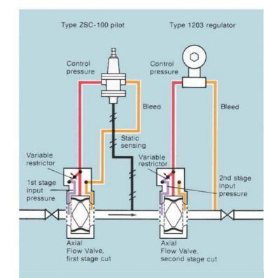
Tow-stage pressure reduction: psi to psi to in. W.C. When large reductions in pressure are required, the cut can be made in two stages. Here an American AFV and Type ZSC-100 pilot control a psi to psi cut. The second stage incorporates a Type 1203 regulator to give a final output pressure in the inches W.C. range.
