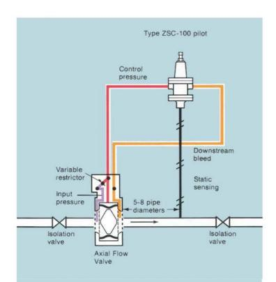
Single-stage pressure reduction. When downstream pressure decreases, spring force increases the effective opening of the pilot. The increase in flow produces a larger pressure drop across the variable restrictor, reducing control pressure to the AFV and increasing flow in the line.
