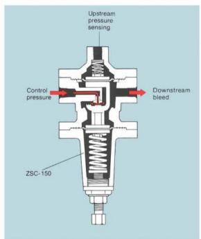
As long as the spring force is greater than the force of the upstream pressure acting on the upstream sensing chamber diaphragm, the regulator is held closed. When upstream pressure increases beyond the setpoint, the regulator opens. Since the exhaust is normally at close-to-zero pressure, a large flow occurs through the regulator, quickly opening the AFV to relieve the overpressure condition.
