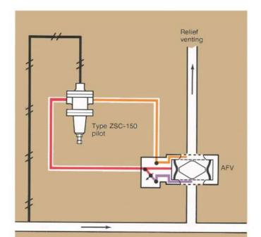
Pressure relief valve. With the ZSC-150 pilot, the AFV is closed as long as upstream pressure is below the setpoint. Because the exhaust port is normally at atmosphere, once the regulator opens, a large drop occurs across the restrictor, causing the AFV to open quickly.
