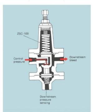
Spring force tends to hold the regulator open. This force is counterbalanced by pressure applied to the downstream sensing chamber diaphragm. When the downstream pressure decreases, the regulator is opened wider, increasing flow. This produces a larger drop across the restrictor and a decrease in control pressure to the AFV, thereby increasing flow to satisfy downstream demand.
