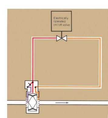
On/off control of flow in a pipeline. When the electrically operated valve is open, the input pressure is bled downstream causing a drop across the restrictor. Since the control pressure is less than the input pressure, the AFV opens to allow flow in the pipeline. Closing the electrically operated valve causes the control pressure to build up to the input pressure, closing the AFV.
