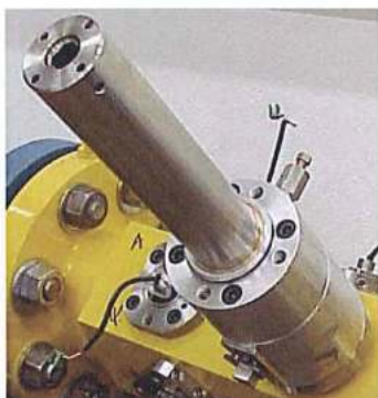
Standard exchangeable transducers under pressure, tool with integrated valve
